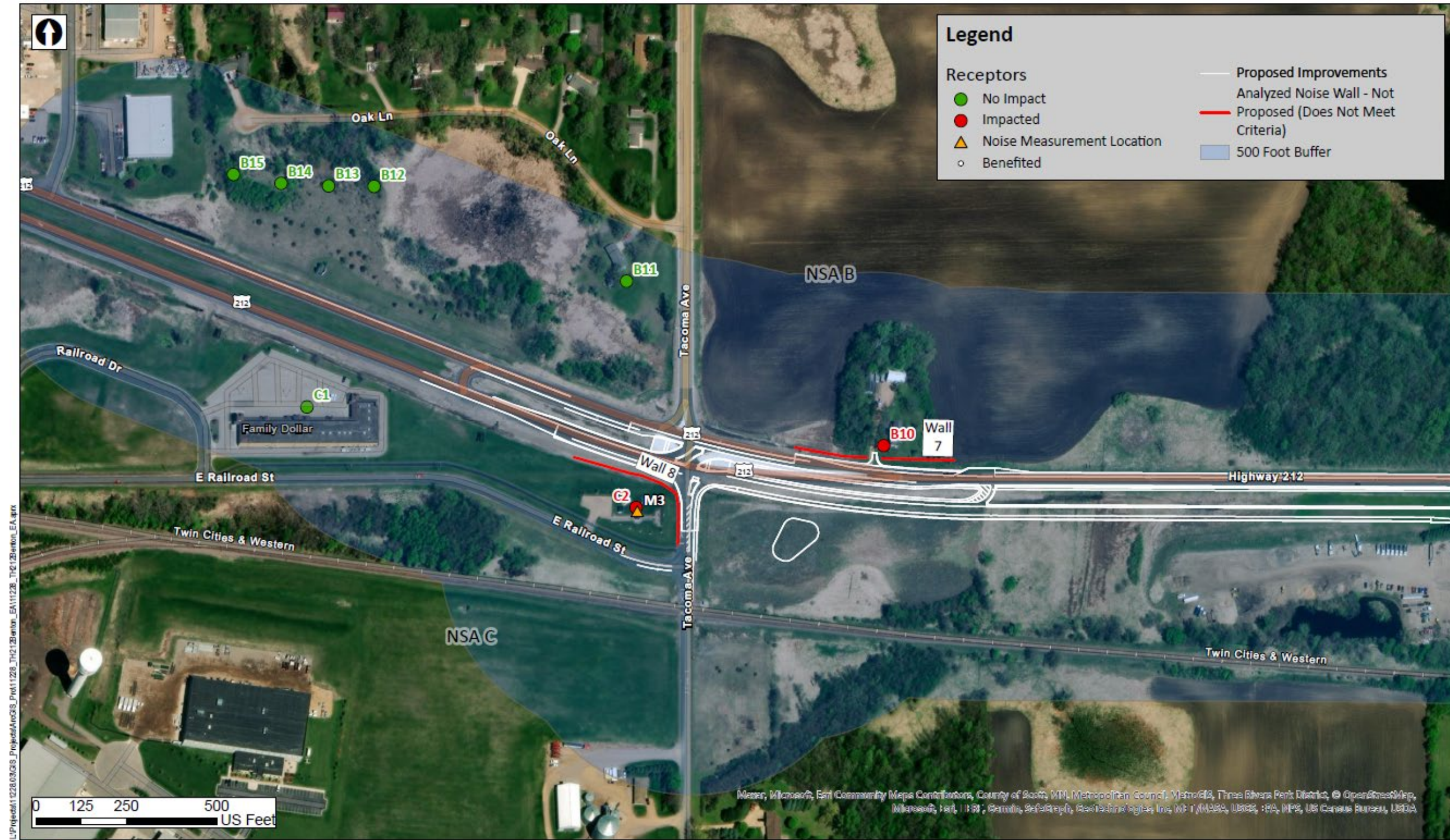
SRF Noise Receptors and Analyzed Noise Wall Locations SP 1013-77 Hwy 212 Benton Township Carver County
