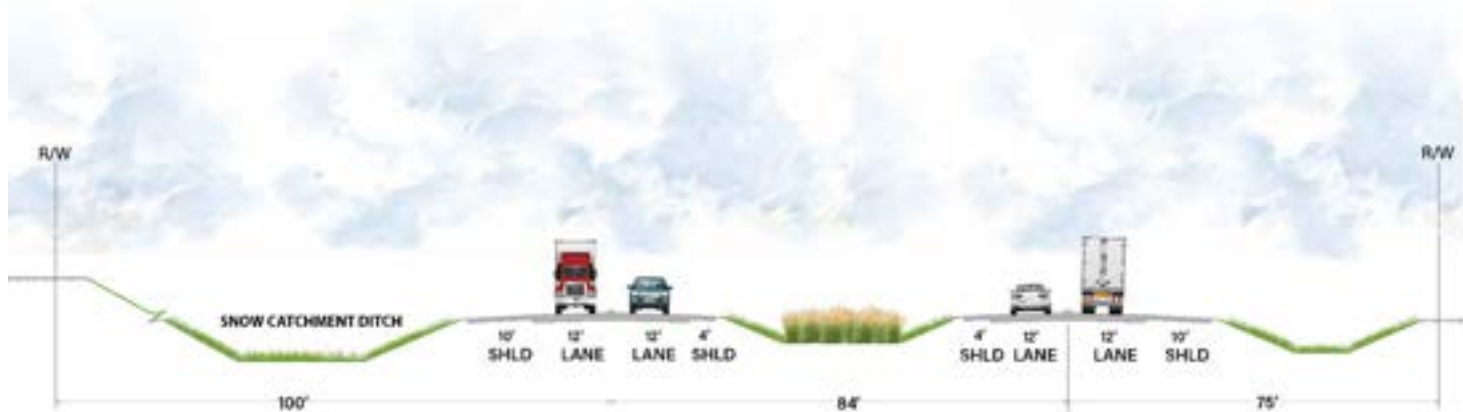
Exhibit 1: Proposed Hwy 212 Four-Lane Divided Highway Section
