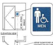
MAC 703.3.10: RESTROOM AND OTHER IDENTIFICATION SIGNS SHALL BE INSTALLED ADJACENT TO THE LATCH SIDE OF THE SHALL BE INSTALLED ADJOCKENT TO THE DITTOR SIDE OF THE DOOR AND THE TACTILE CHARACTERS SHALL BE 48 INCHES MINIMUM ABOVE THE FLOOR MEASURED FROM THE BASE OF THE LOWEST TACTILE CHARACTER AND 60 INCHES MAXIMUM ABOVE THE FLOOR MEASURED TO THE BASE OF THE HIGHEST TACTILE
