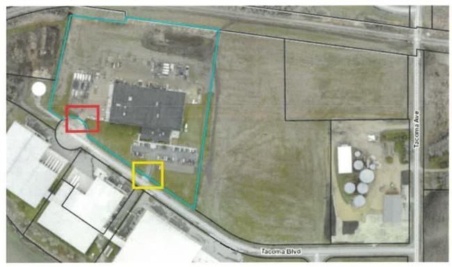
This Site Plan Review has been requested to approve a reconfiguration of truck access to the campus. The reconfiguration would allow trucks to enter from a new access off of Tacoma Ave., and exit from a second newly created access on to Tacoma Blvd. This change would eliminate on-street truck parking and staging on shipping days, keeping operations entirely contained on the Sackett Waconia Campus.
